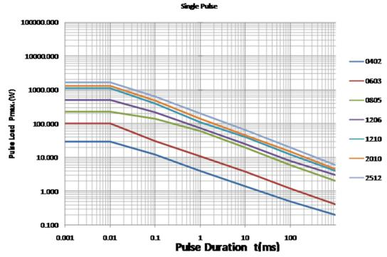
Single-pulse high-voltage overload test:
