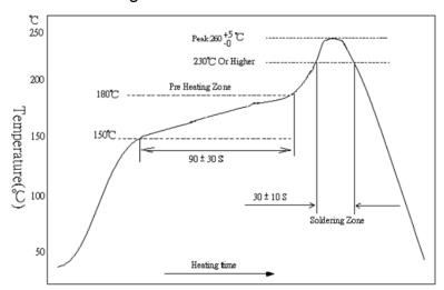
Remark: The peak temperature of soldering heat is 260 +5/-0 °C for 10 seconds
